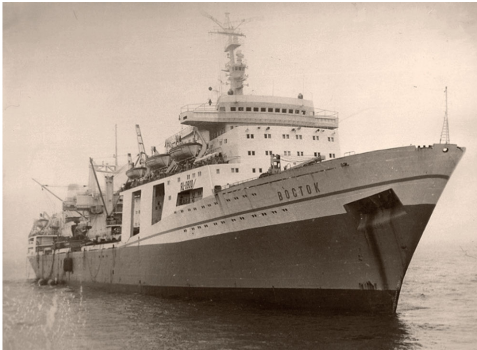
Figure 3. A Soviet mother ship. The Soviet vessel Vostok , 'Восток' (IMO 6915805) built in 1971, with homeports in Odessa and Vladivostok, was the largest of all mother ships ever constructed at the time. She measured 225 m in length and had a capacity to produce 150 000 cans and to freeze 200 tons of fish per day. The vessel contained a movie theatre and swimming pool [39]. She was scrapped around 2002 [40]. Photo: Gena Anfimov.
