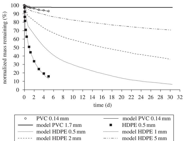
Figure 5. Comparison of *o*-xylene desorption data and one-compartment diffusion model fits as well as predictions of *o*-xylene desorption rates from PVC and HDPE spheres of different diameters. Desorption data were measured after six months of equilibration in ultrapure water.
