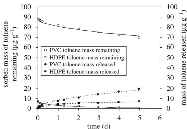
Figure 6. Effect of polymer type on sorbed toluene mass remaining and released per gram of sorbent. Lines represent model fits for sorption equilibrium liquid-phase concentration ( $C_e$ ) of  $100 \mu\text{g l}^{-1}$ ,  $K_p = 70.7 (\mu\text{g kg}^{-1})(\text{l } \mu\text{g}^{-1})$  for HDPE and  $K_f = 1663 (\mu\text{g kg}^{-1})(\text{l } \mu\text{g}^{-1})$ , and  $n = 0.864$  for PVC (Wu *et al.* 2001). The particle diameters of HDPE and PVC were 0.5 and 0.14 mm, respectively.
